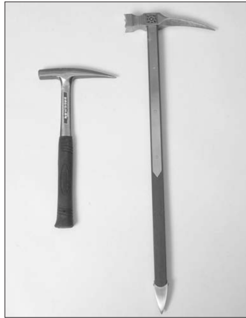
MODERN ROCK PICK AND MEDIEVAL WAR HAMMER. THE ROCK PICK IS ON THE LEFT. NOTE THAT THEY ARE SIMILARLY CONSTRUCTED.
